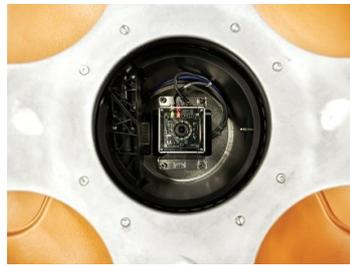
**Figure 2.** Navigation System of Kiva Robots (Source: Guizzo, E. ,2008)
