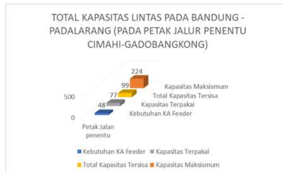
Figure 2 Total Capacity on the Bandung-Padalarang Crossing
