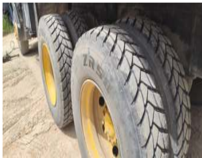
Figure 13: Tipper Dumper with multiple balding tires
