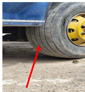
Figure 13: Tipper Dumper with multiple balding tires
