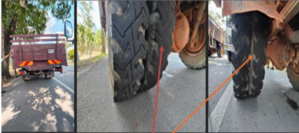
Figure 11: Small Lorry inner axel balding
