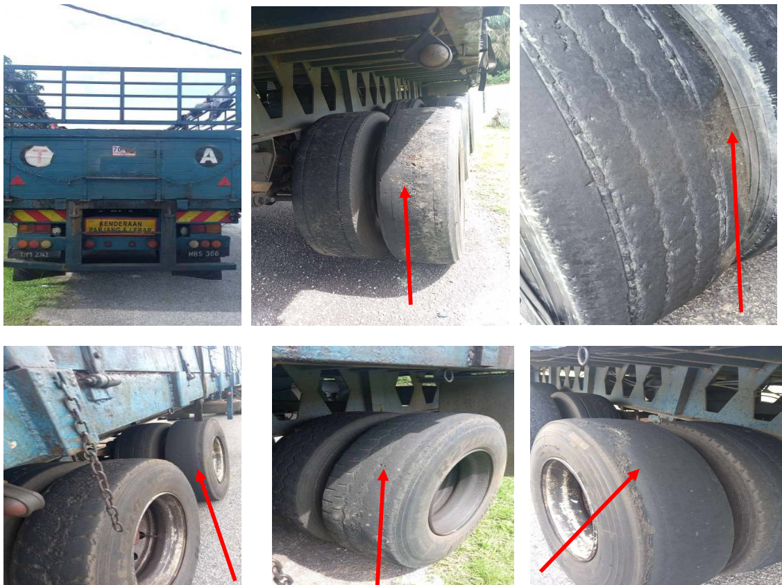
Figure 12: Semi Trailer with multiple worn out tires
